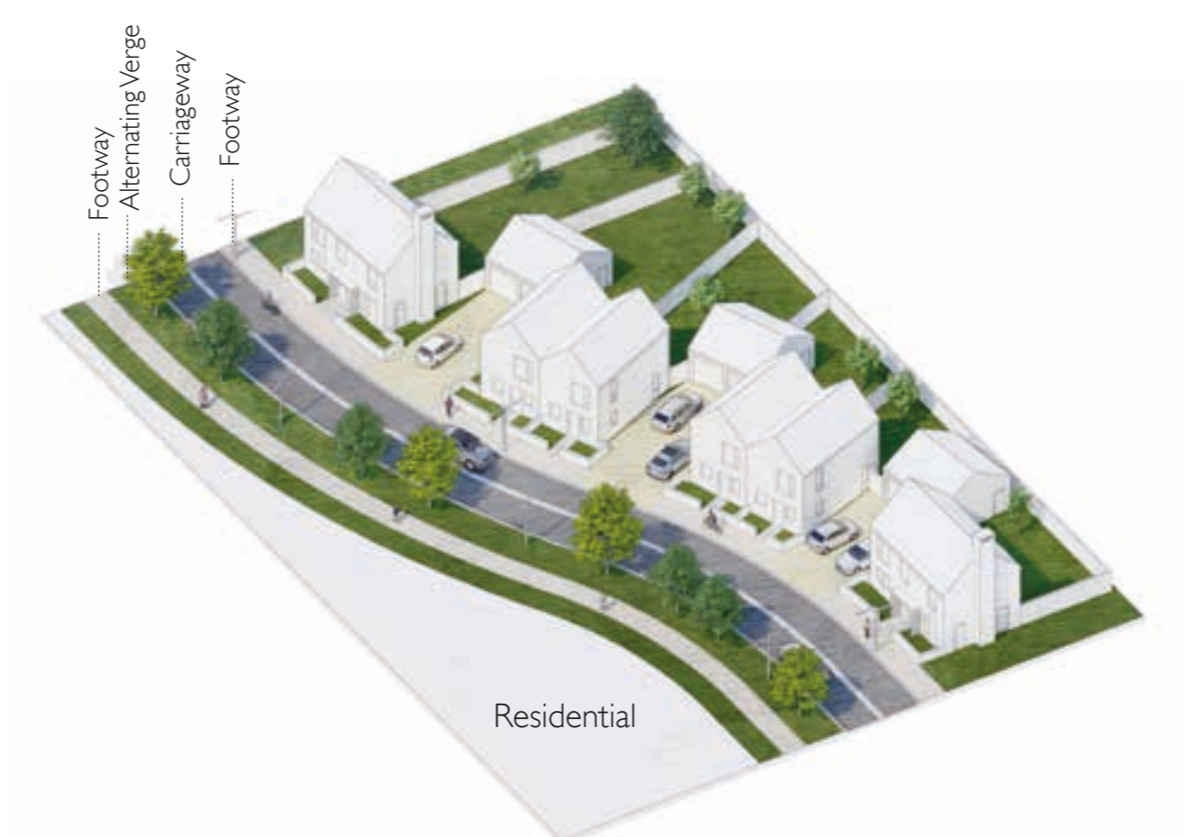
Illustrative axonometric of Compasses Way (Type B)
